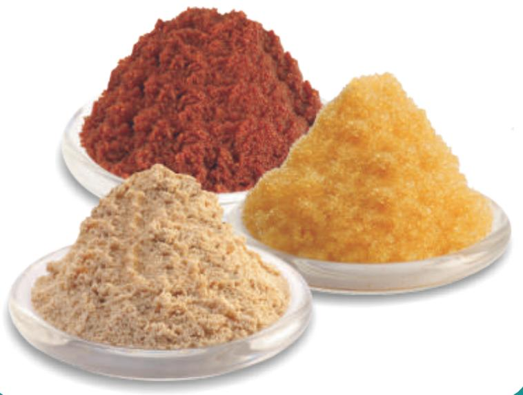
Ion Exchange Resins or Ion Exchangers were invented for meeting the needs of the industries so as to ensure water of high quality that meets the stringent effluent limiting conditions of new age turbines and boilers are achieved.
